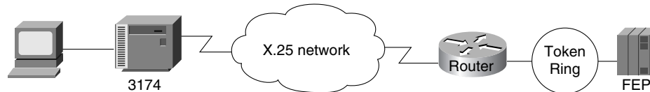
Figure 5-18 Simple topology for QLLC conversion.
